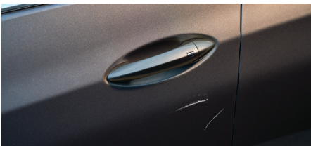
1 dent or 2 scratches (less than 4”) per panel
