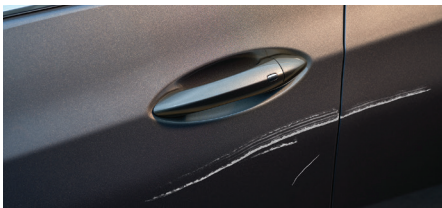
1 dent or 2 scratches (more than 4”) per panel
