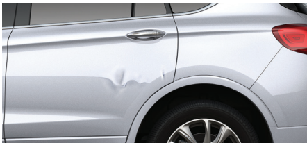
Hail damage or punctures on any panel
